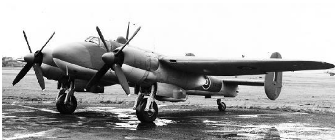
DX255, the second armed prototype – the fastest fully armed bomber of its day at 355 mph - and below, KV370 without nose machine guns. When hostilities ceased, there were unarmed conversions to passenger-carrying communications versions, the C.1 and C.2.
