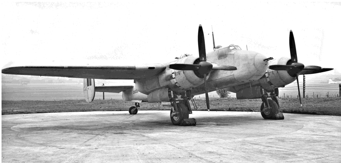
DX255, the second armed prototype – the fastest fully armed bomber of its day at 355 mph - and below, KV370 without nose machine guns. When hostilities ceased, there were unarmed conversions to passenger-carrying communications versions, the C.1 and C.2.
