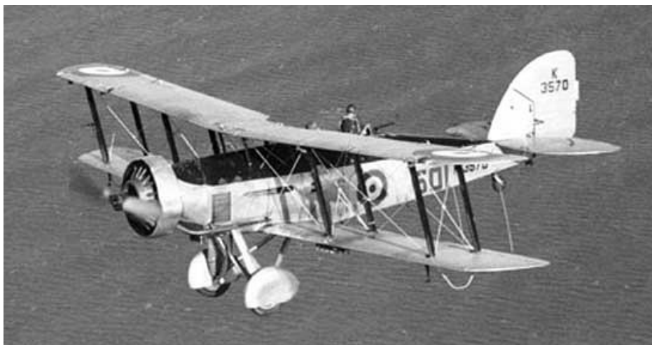
A 501 Squadron Westland Wallace Mk.1 powered by a 680 hp Bristol Pegasus IIM3 9- cylinder radial piston engine c. June 1936.
