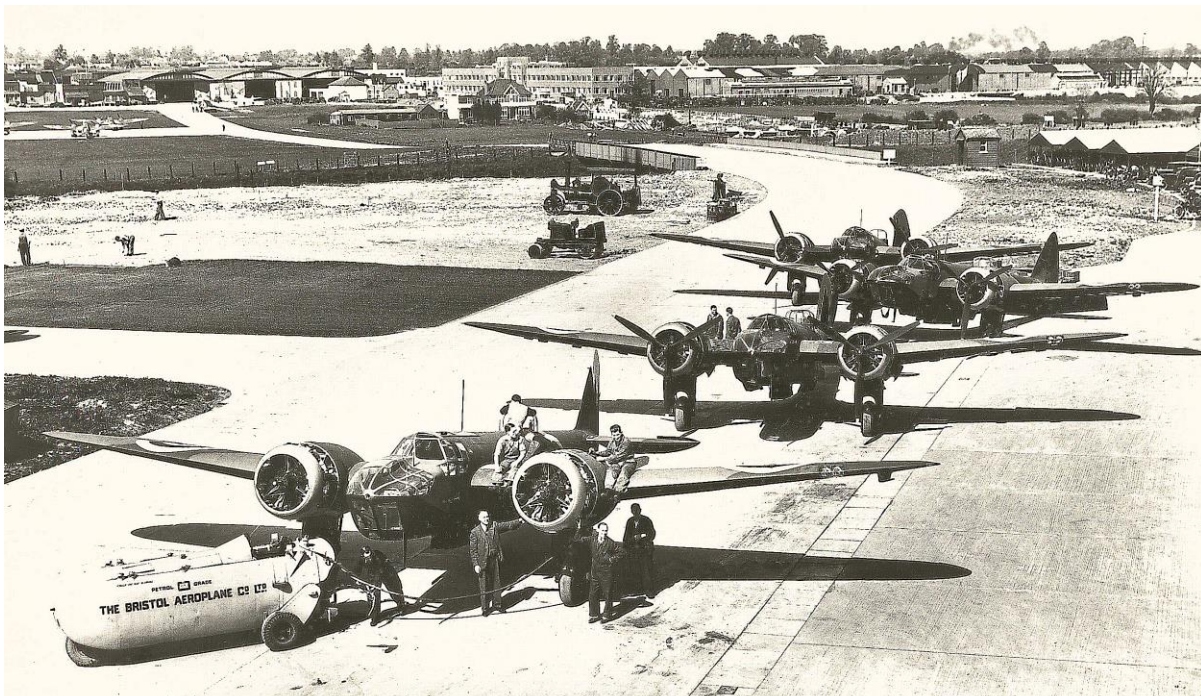
Filton, Summer 1938. A wealth of detail can be seen in this photograph of a flight of Blenheim Mk.IV aircraft just returned from ground testing. The leading aircraft has already had its propellers removed prior to be put into No.1 Flight Shed and is about to be defueled – both precautions against accidents whilst being worked on in the hangars. The former flying school hangars, by now the West Works of the Engine Division, can be seen in the background (in 2020 this is the site of the GPO Sorting Office) with the new hard runway and taxiways leading to the bridge over the GWR cutting, under and to the left of which were the Filton West platforms. A hard standing is being built south and west of the railway bridge, on which aircraft on test and awaiting delivery would be parked. In 2020, it is underneath Airbus buildings and car park. To the top right can be seen the 1930's office building of the Engine Division and the Filton Engine Shadow Factory bicycle sheds and bus station – the factory is out of the picture to the right.
